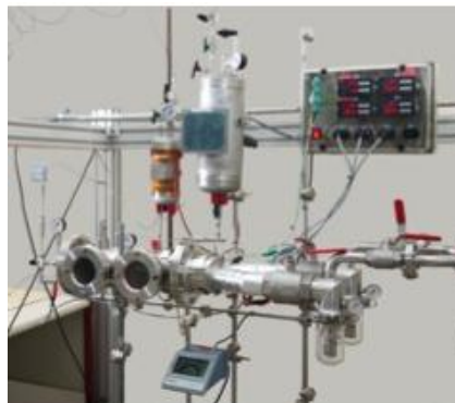
Figure 1: Spray Flash Evaporation (SFE) pilot plant.
